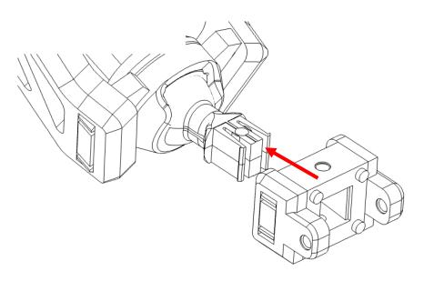
Lock the adaptor to the mount using the included LEGO 3L pins
