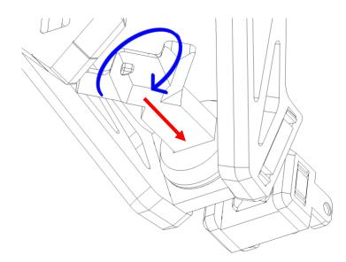
Place the set onto the wall mount as shown and use the ball joint to position the set to your liking. Then tighten the ball joint cap using the included wrench.
