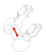
Assemble the ball joint as shown and tighten the cap finger tight
