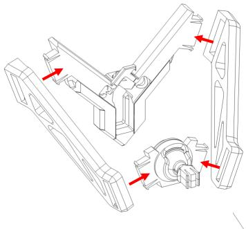
If wall mounting, install the wall plugs with 45mm spacing, then fit the mount using the screws. Do not use a power drill to screw the screws. Please use a screw driver.
