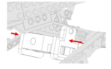
Insert the adaptor clips into the 3D print and the technic pin (both sides)
